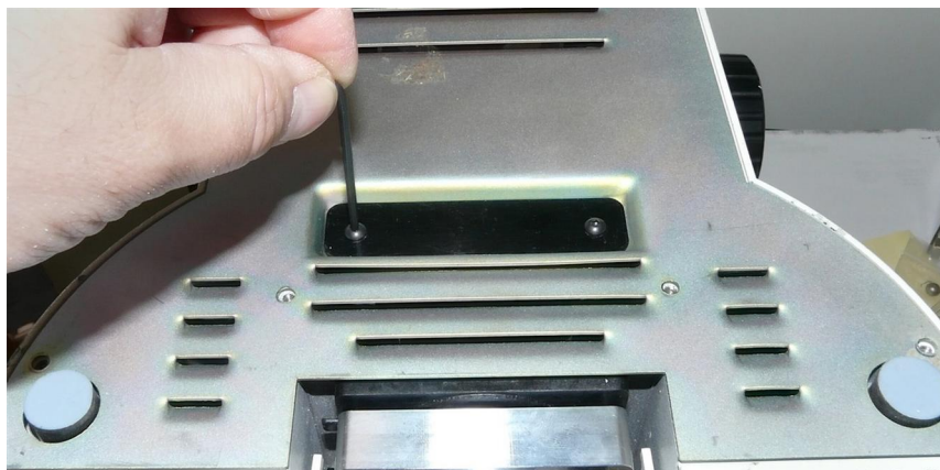
(3) Replace the bottom cover and tighten the black screws for holding the filter. (use a 2mm hex key)
