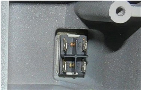
(1) Unscrew the obsolete AC power bracket and pull it away from the microscope.
