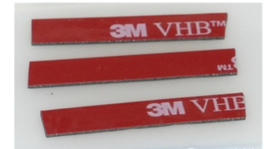
Tape to secure wires.
