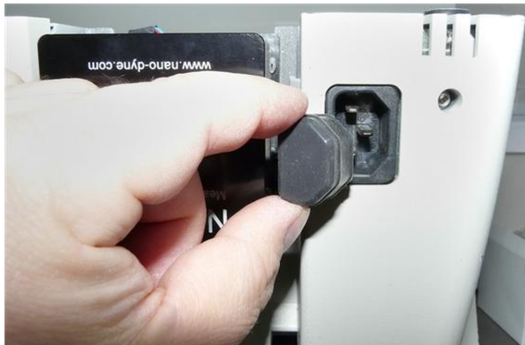
(5) Install the silicone rubber AC blocking plug provided.
