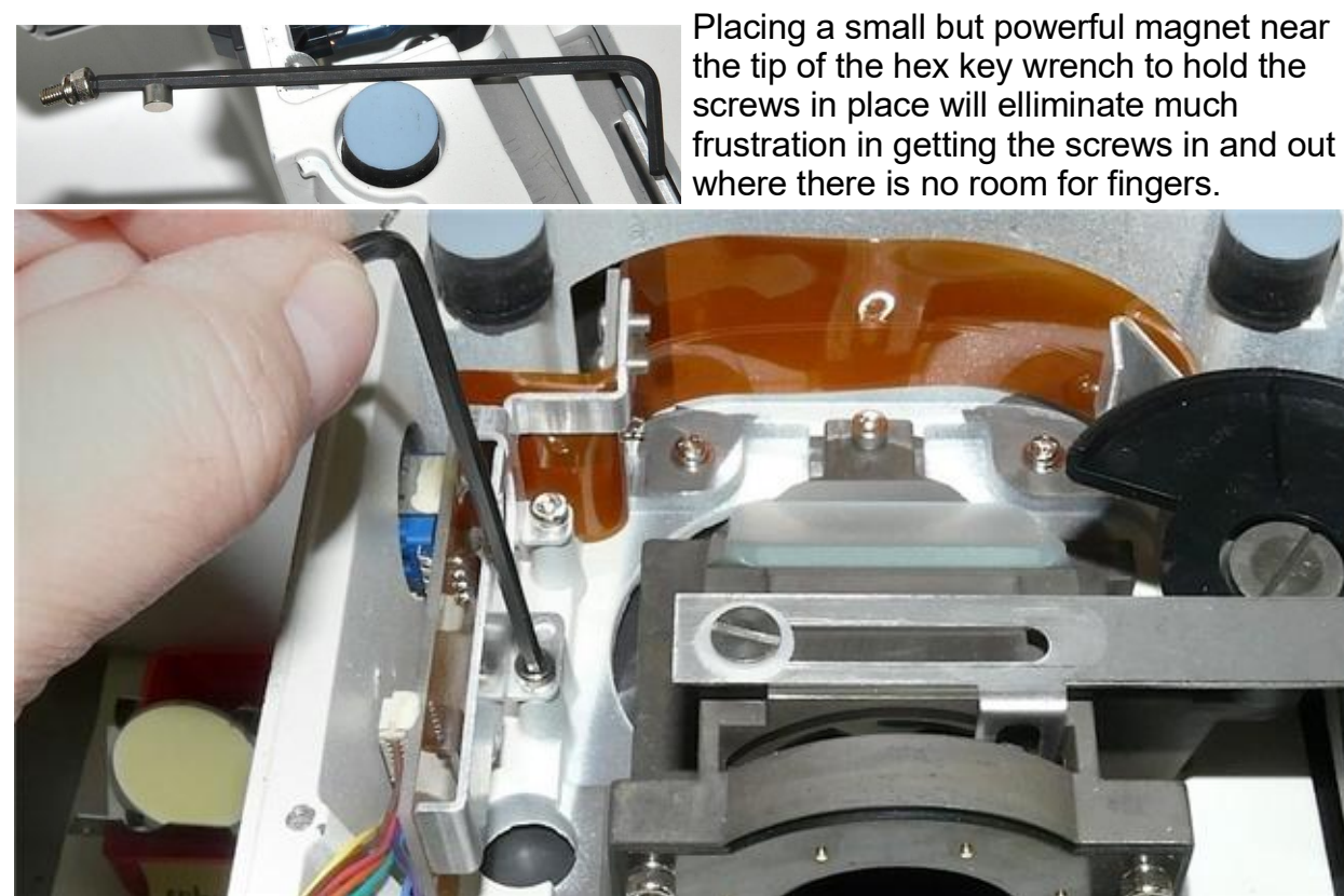
(4) Remove the mounting screws for the pot plate PCB.
