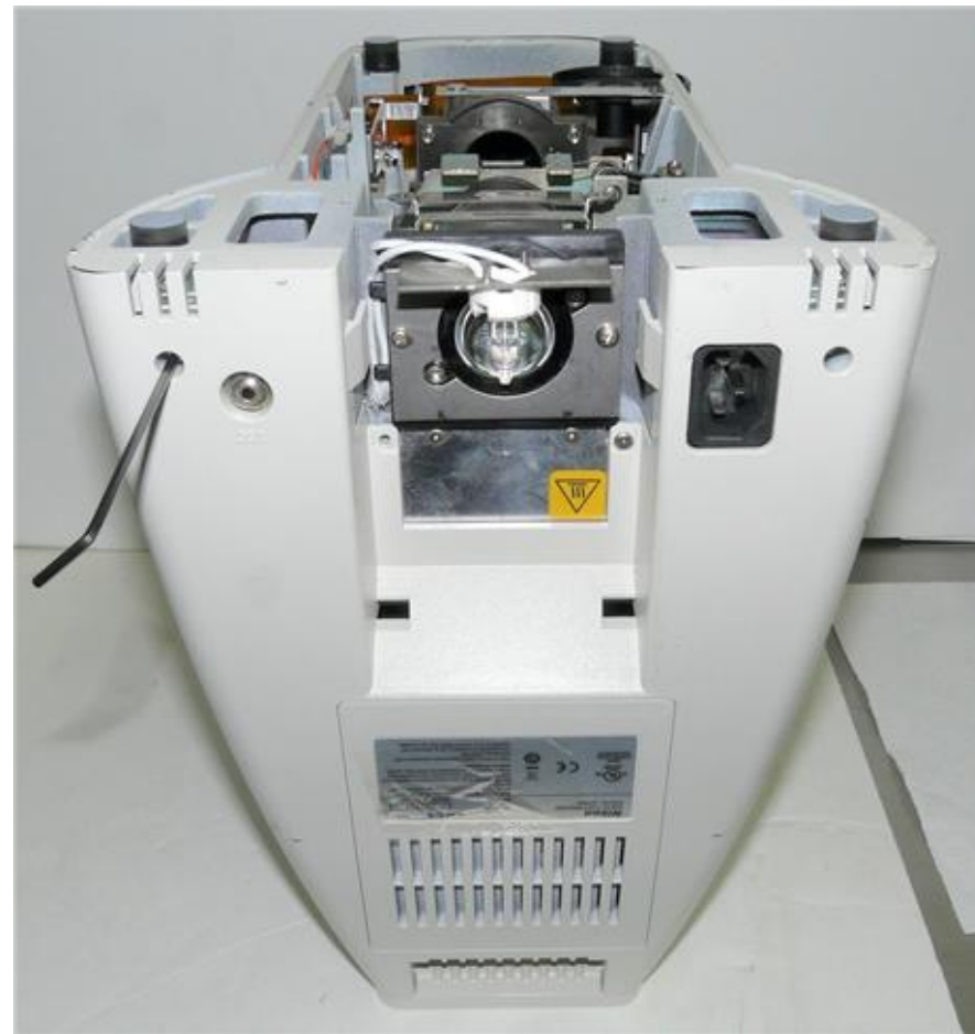
(4) Remove the back cover (6 screws).
