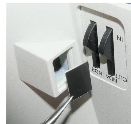
(6) Install the blank-off plate in place of the power switch. Press firmly in place.
