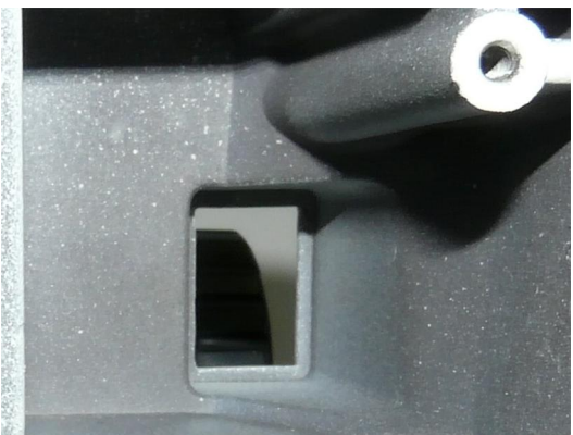
(4) Remove the power switch. Use tweezers or a small screw driver to compress the plastic retainers holding it in place while pushing it out.
