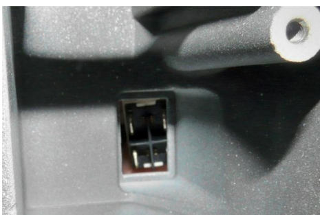
(1) Unscrew the obsolete AC power bracket and pull it away from the microscope.
