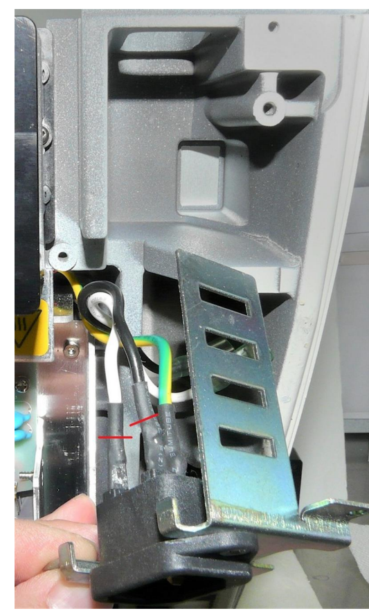
(3) Cut the white and black AC power leads at the red lines in the above photo and discard the AC wires. Replace the AC power receptacle.
