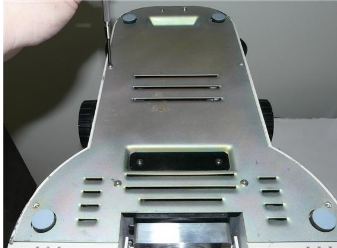
(4) Install the rest of the screws. The two just under the black filter holder need a 1.5mm hex key. The other 6 need a phillips screwdriver.
