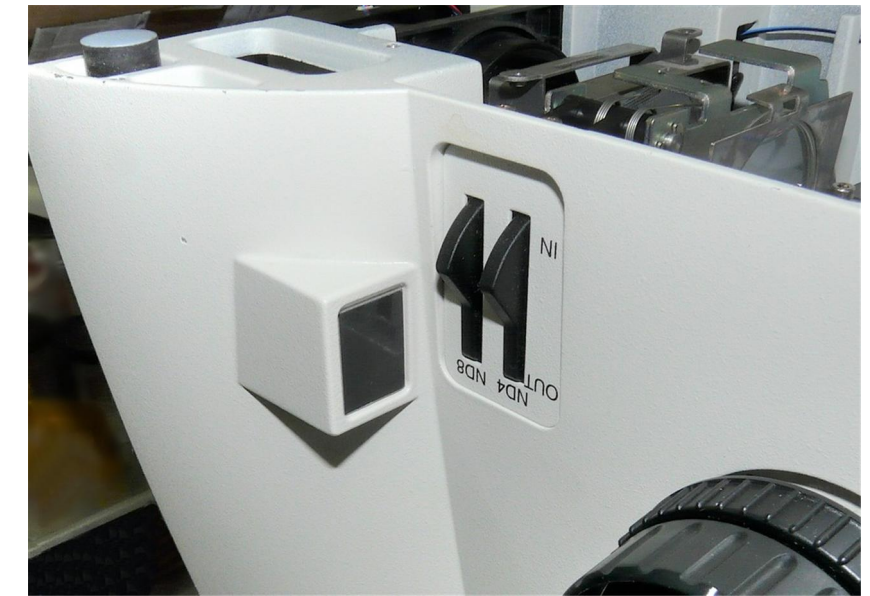
(7) Blank-off plate installed in microscope.
